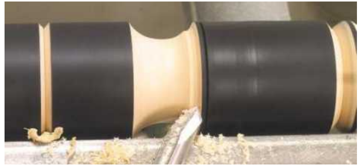
▲ Pic.8 You must keep your right hand low through the cut; this will allow the bevel to rub. If you're not getting a good finish, it's often because the tool is too horizontal
